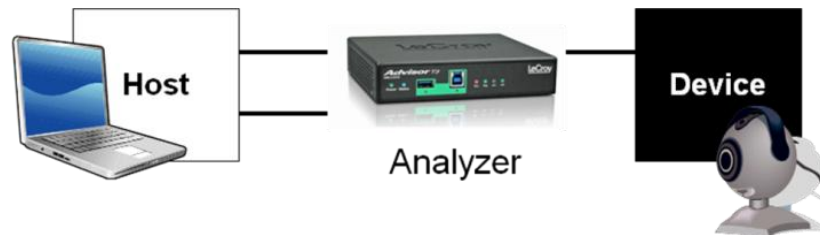
Figure 52. Using Analyzer with Single Host
