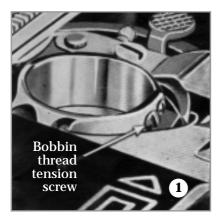
(1) The bobbin has a small spring on its case, which delivers the thread under a slight tension.
