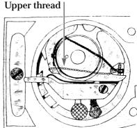
Accurate synchronisation (or timing) between the simultaneous tasks of stitch formation is essential for the machine to work.
