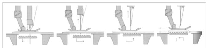
While the needle and thread penetrate the fabric, the feed dog is still and the fabric is held between the presser foot and the throat plate, keeping it taut.
