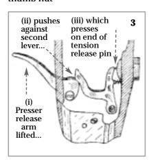
(3) The upper tension is released completely when the presser bar lifter is raised. The lifter presses on a pin which in turn pushes the discs apart.
