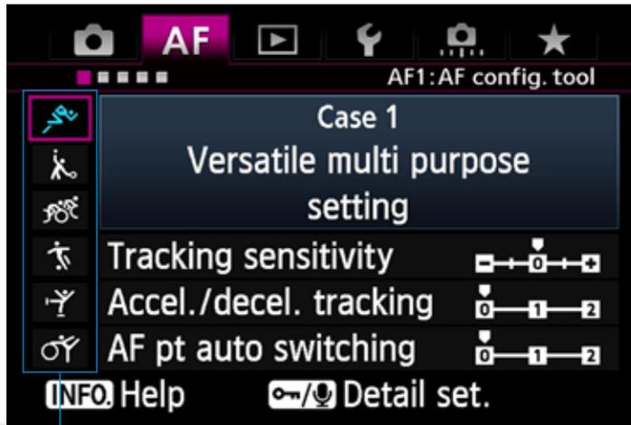
[AF1] tab screen. By selecting an appropriate preset from the Case 1 - Case 6 icons on the left side of the screen, the most effective AI Servo AF settings for different subjects can be made.
