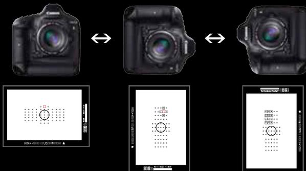
First, select [Select separate AF points] from [Orientation linked AF point]. Next, select the AF area selection mode and the manually selected AF point for each of the positions (orientation) of A) Horizontal position, B) Vertical position with grip at the top, and if required C) Vertical position with grip at the bottom. The settings will automatically be remembered. Now, for each of these orientations the camera will automatically switch to the select mode and AF points.
