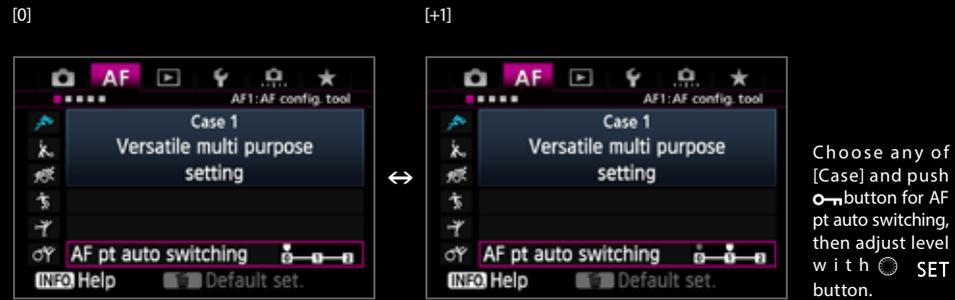
The [AF pt auto switching] parameter is used for setting characteristics of AF point switching when the subject has a lot of movements. This parameter is only for switching between multiple AF points, so it is unavailable when using AF area selection modes [Single-point Spot AF] and [Single-point AF]. The [0] setting is a standard setting for moderate switching of AF points. The [+1/+2] settings are used when shooting subjects with erratic movement which
