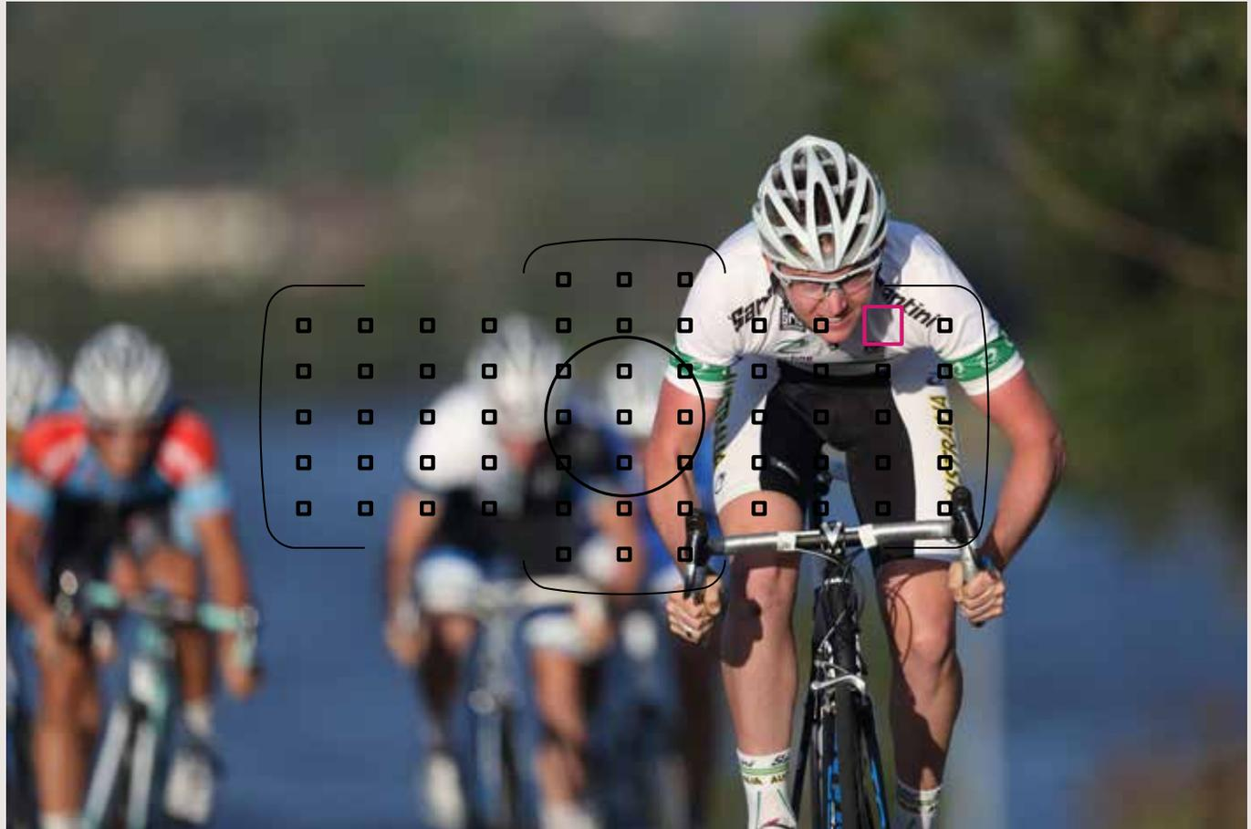
When using [Auto selection of 61 AF points] during [AI Servo AF], focusing will start from the manually selected AF point, the camera will automatically change the AF point selecting from all 61 points as the subject moves. The AF points are arranged in a wide area so it is useful for capturing and tracking of subjects, however,
