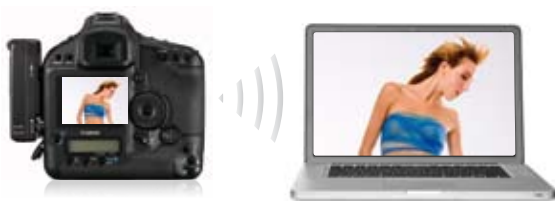
Remote Live View renders the real-time sensor image on the computer.
