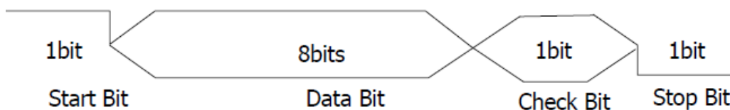
Figure 5-13 RS232 Protocol Schematic Diagram
