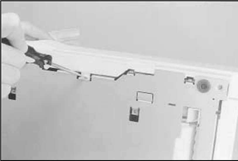
Figure A-8 Latch Location on Underside of Duplexer
